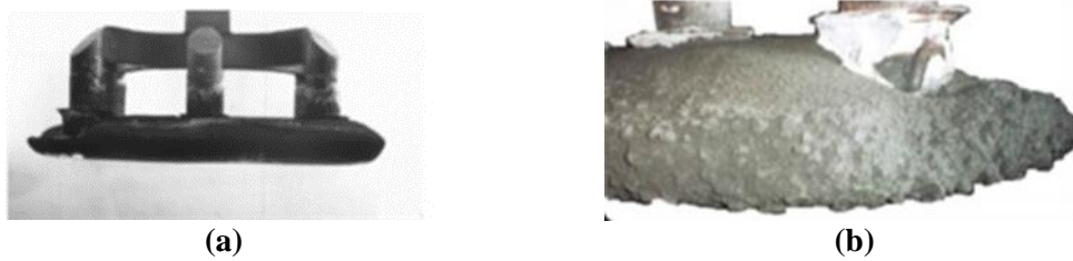
Figure 2. Images of (a) anode butt with pin attack and (b) anode butt with excessive reactivity.
